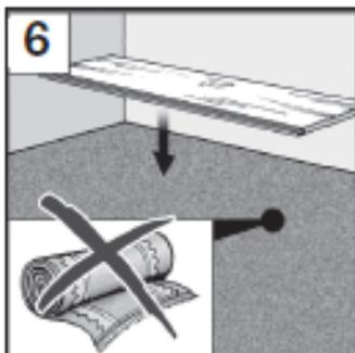
Carpeting, foamed PVC floor coverings and all types of foam must always be removed [6] as they are not suitable as subsurfaces. Walking on the floor surface may otherwise cause a springy movement in the flooring and too much pressure in the edge areas, which can result in the formation of gaps. Carpeting must also be removed for hygienic reasons. Moisture can lead to the formation of mould and bacteria.
